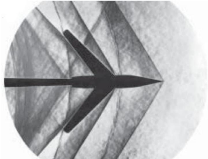
Schlieren photograph of an attached shock on a sharp-nosed supersonic body.
