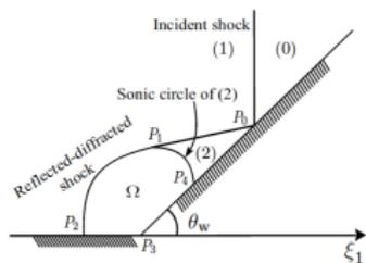
FIGURE 3. Supersonic regular reflection-diffraction configuration [8].
