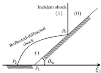
FIGURE 4. Subsonic regular reflection-diffraction configuration [8].
